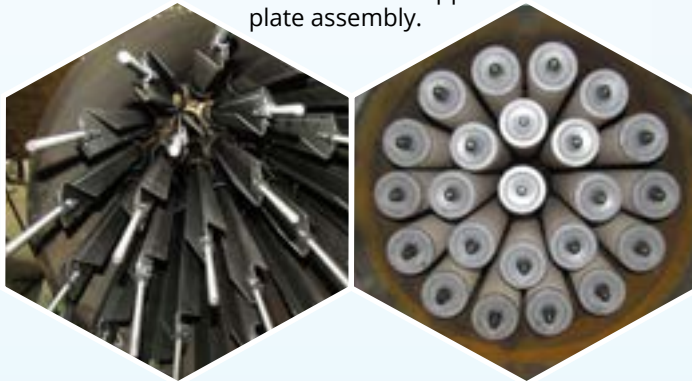
Elements mounted on completed riser assembly.
